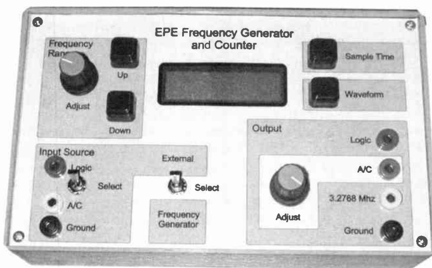
Fig. 1. Front panel of the author's Frequency Generator and Counter case.
