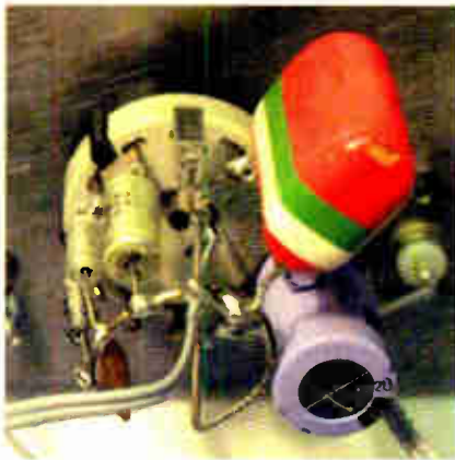
Frequency range capacitors mounted directly on the switch tags.
