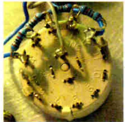
Amplitude range resistors mounted directly across the switch tags.
