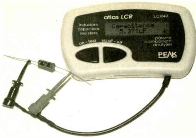
Checking-out the value of a suspect electrolytic capacitor.
