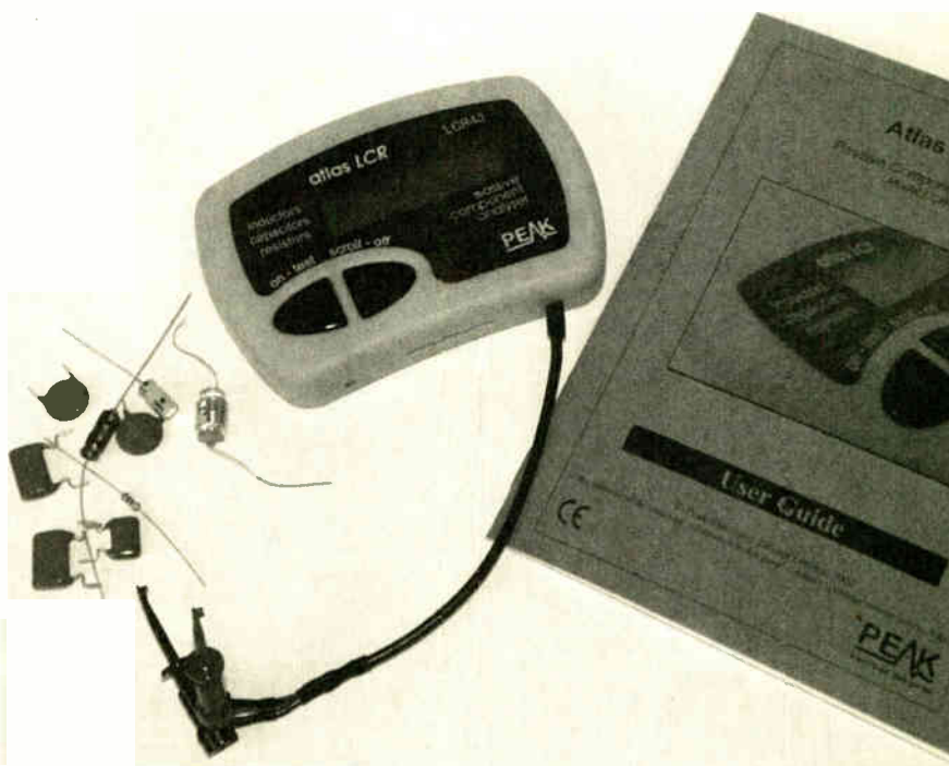
The Atlas LCR Passive Component Analyser from Peak Electronic Design.
