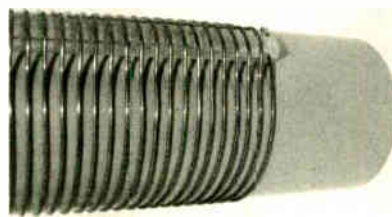
Acrylic spacer strip holds winding proud of the former to permit tapping.
