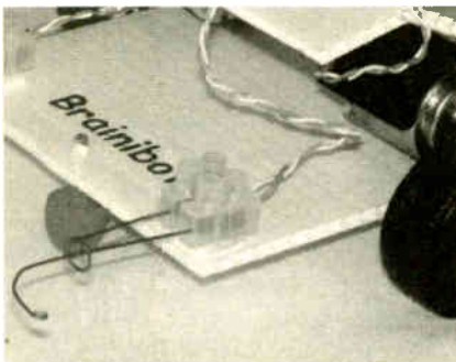
An antenna mounted in terminal block.
