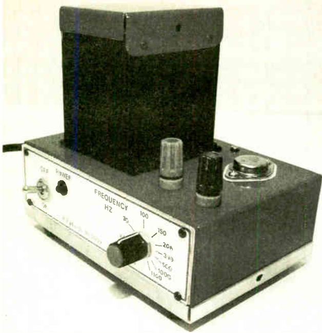
The completed Power Supply and Pulsing Unit showing the "shroud" protecting the mains transformer.
