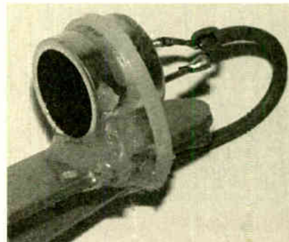
Transducer secured to probe mount using a cable tie and hot-melt glue.
