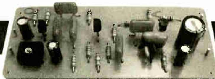
Bandpass Filter printed circuit board.
