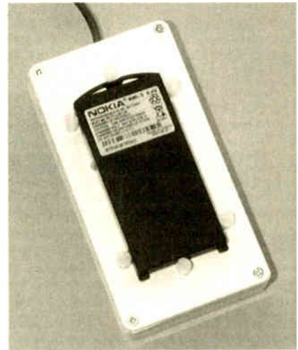
The mobile phone battery mounted on the battery holder contact box, between the locating pegs.
