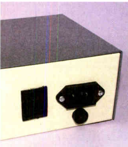
Rear-mounted male mains connector, mains switch and fuseholder.
