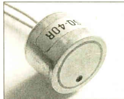
The author's "touch-switch" was made from a broken ultrasonic transducer.
