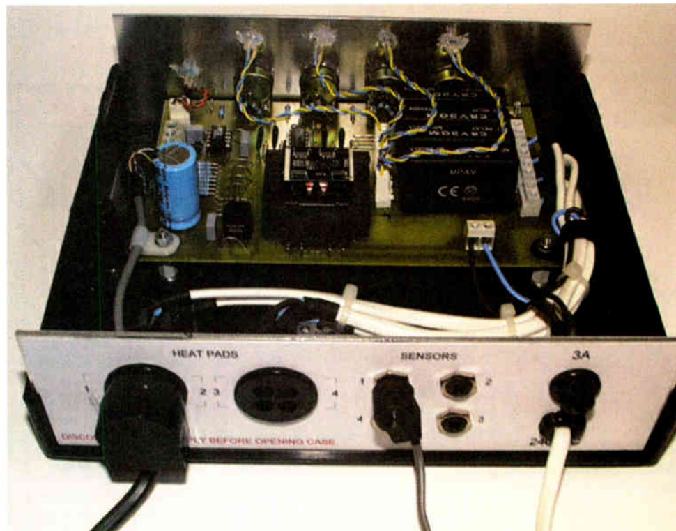
The rear panel sockets, fuse and mains cable positioning.
