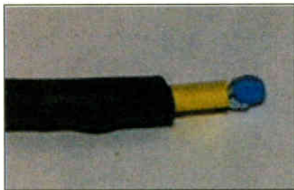
Make sure the thermistor leads are fully insulated.
