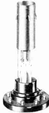
Fig. 1.—THE COSSOR CATHODE RAY OSCILLOGRAPH.
