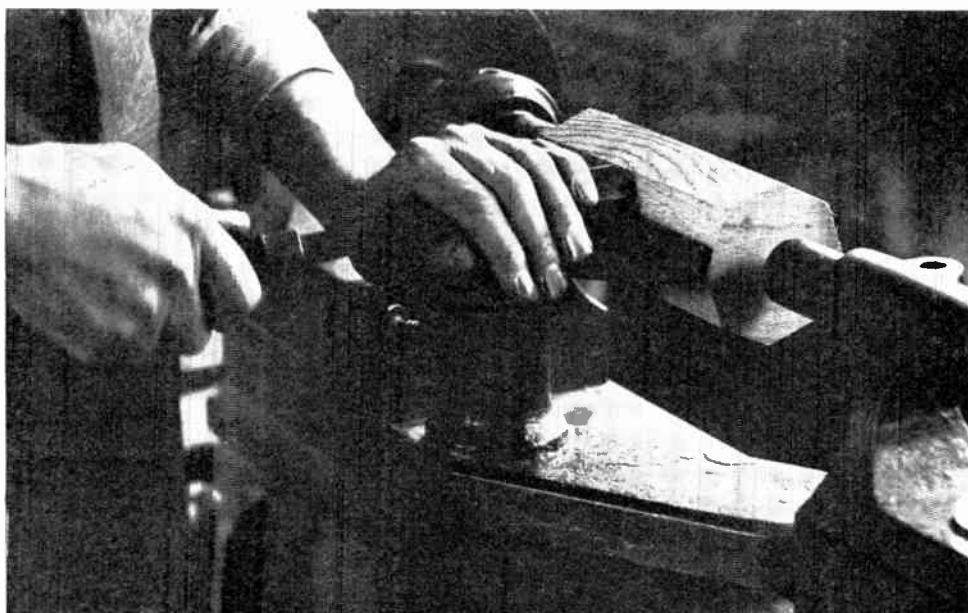
Fig. 7. —TURNING THE LOWEST SECTION OF THE SHAFT D.
