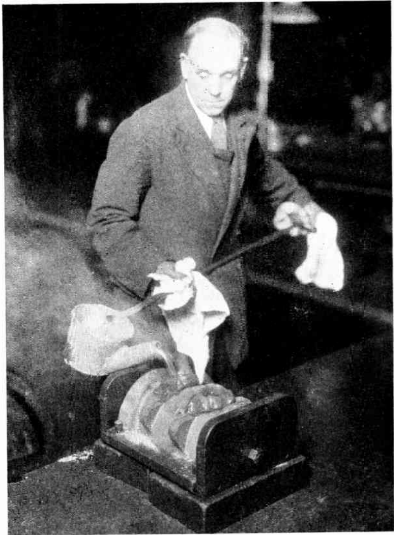
Fig. 15.—POURING A HALF BEARING.
