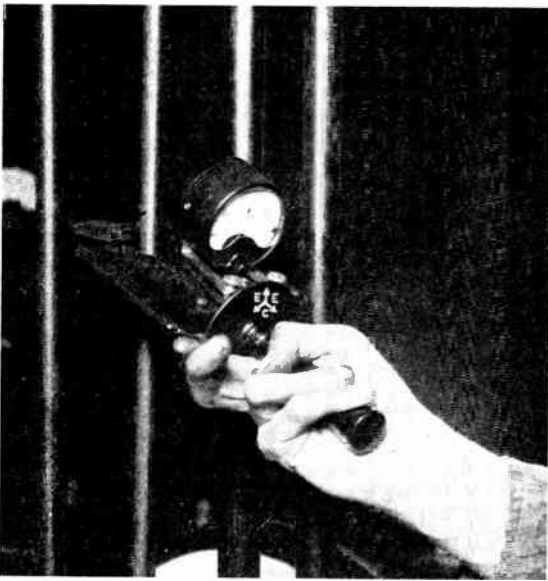
Fig. 27.—AMMETER WITH HINGED CORE TRANSFORMER CLAMPED ROUND A CONDUCTOR CARRYING A.C. AND INDICATING THE VALUE OF THE CURRENT. The instrument shown has two ranges, 0-100 amperes and 0-500 amperes.
