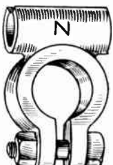
Fig. 17.—CONVENIENT TYPE OF BATTERY TERMINAL FOR MOTOR-CAR BATTERY.
