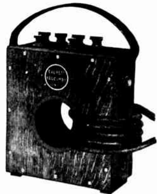
Fig. 25. —OMNI-RANGE CURRENT TRANSFORMER, WITH VARIOUS RANGES UP TO 1,000 AMPERES. As shown (with five turns), the ratio is 200/5 amperes.
