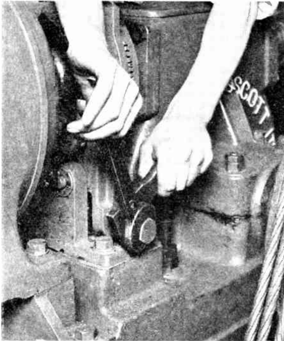
Fig. 15. — ADJUSTING THE SPRING PRESSURE.
