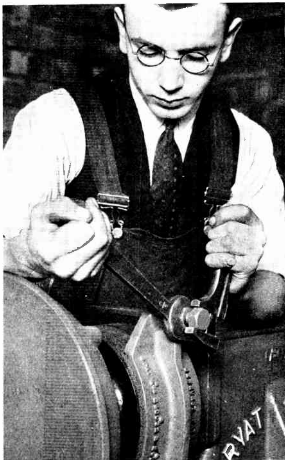
Fig. 14. —ADJUSTING THE AIR GAP OF THE BRAKE ARMATURE.
