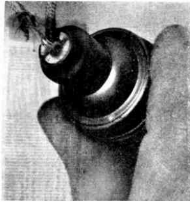
Fig. 12.—SHOWING WORN FLEX. A frequent cause of a blown fuse.
