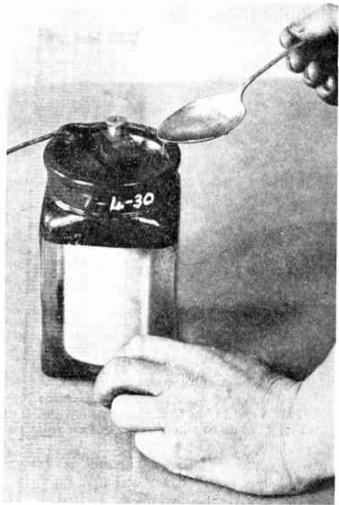
Fig. 5. —HOW TO ADD WATER TO A CELL.
