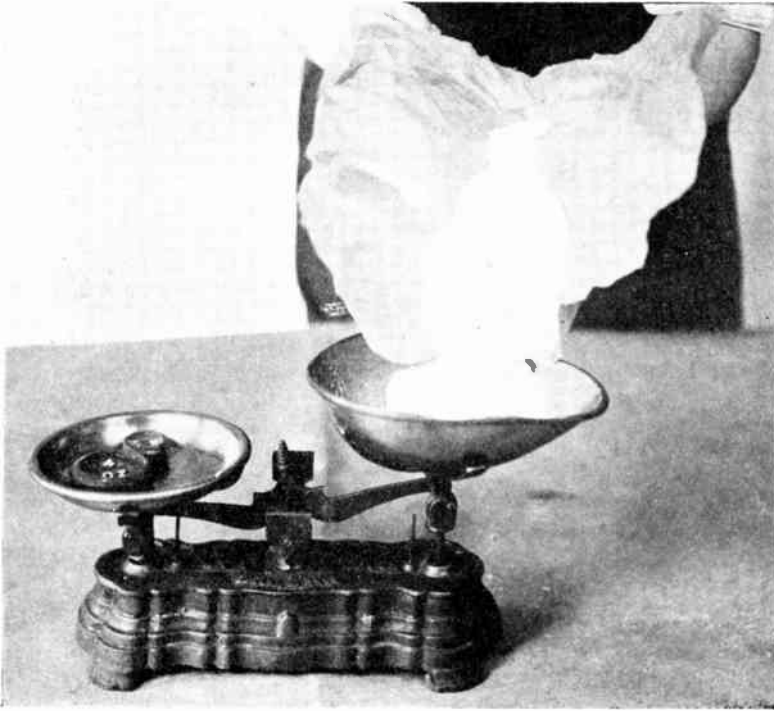
Fig. 2. —HOW TO WEIGH UP SAL-AMMONIAC CRYSTALS.
