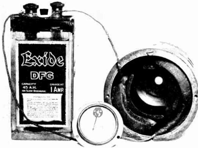
Fig. 13.—TESTING FIELD WINDING FOR CONTINUITY.
