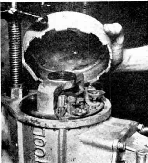
Fig. 15. —REMOVING THE TOP COVER OF AN ELECTRIC TOOL.
