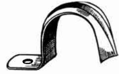
Fig. 14.—ORDINARY SADDLE. For holding conduit in angles.
