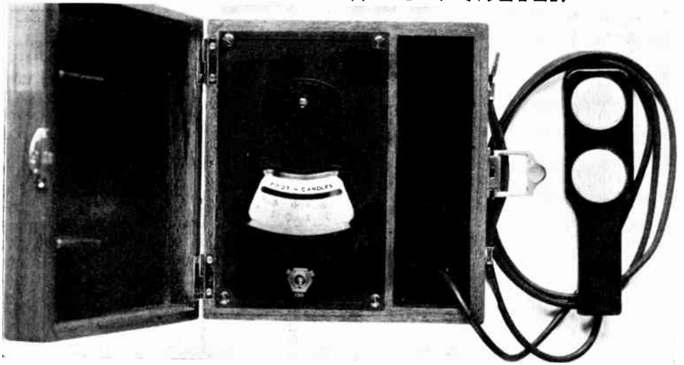
Fig. 1.—THE WESTON PORTABLE ILLUMINATION METER.
