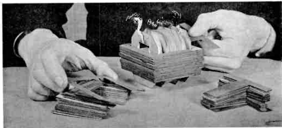
Fig. 9.—FITTING THE CORE WHEN MAKING THE TRANSFORMER.
