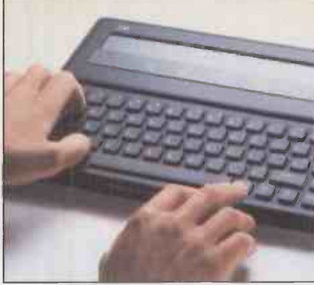
Full QWERTY keyboard offers 'silent', moving short-travel keys. Foldaway foot raises the Z88 12 1/2" for comfortable viewing and typing.
