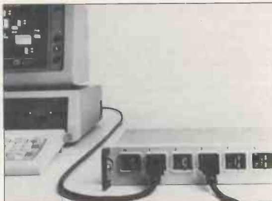
The multi-station access unit of the Token Ring network provides a central control point for maintenance.
