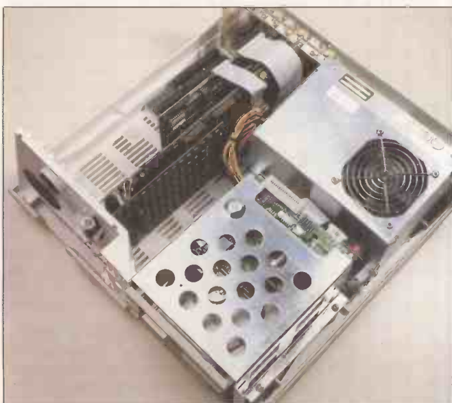
Above: Most of the circuitry is hidden under the power supply. Right: The motherboard houses a socket for an 80387. Four of the expansion slots are fitted on the daughter board.
