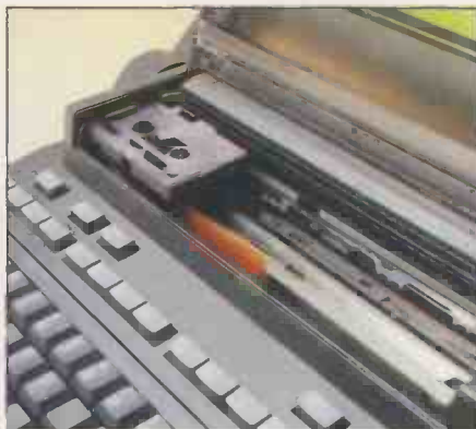
Hard disc and printer (below) are built in, but to load from a floppy you need an external drive (inset).
