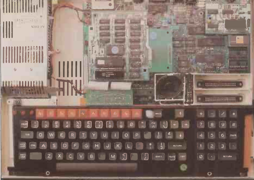
Above: The Econet interface plugs into two connectors located at the top right-hand corner of the PCB. The large white connector on the left of the PCB allows a modem or other internal add-ons to be attached, though the limited cooling within the case is a restriction.
