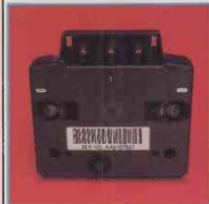
Because of its unusual geometry the Penman's body executes a curve even when drawing a straight line. The white slits are the paper edge detectors.
