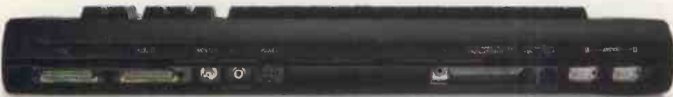
Input/Output Monitor, Hi-Fi, Power, TV, Centronics, Cassette Mic and Ear, and two Joystick ports all come as standard; the twin RS232 ports are available as expansions.
