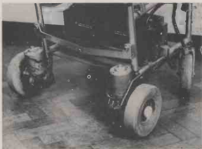
Picture 3: Standard wheelchair layout with driving wheels at the rear, as used on the University of California's 'JASON'.
