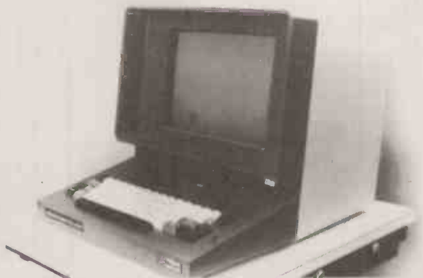
PERKIN ELMER 550 BANTAM, Teletype compatible Visual Display unit.
