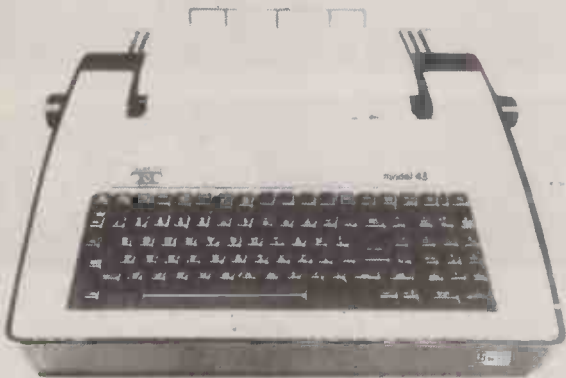
TELETYPE MODEL 43 10/30 C.P.S. Keyboard send/receive terminal.
