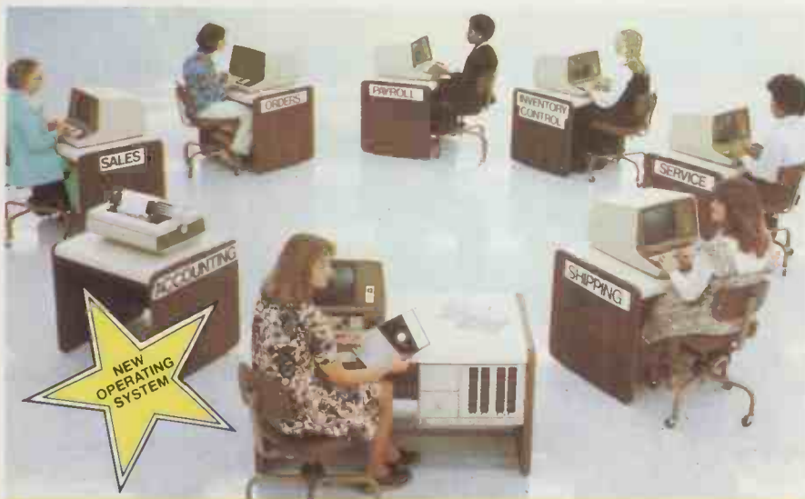
Multi-user System Three, with 320K memory, 4 discs, 7 terminals and fast line printer. Each terminal has its own operating system, and can run any software package independently.
