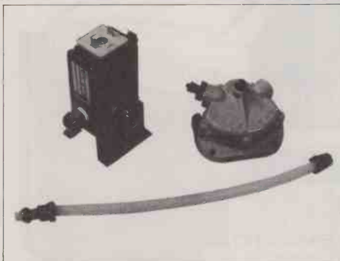
Picture 7: Fluid drive motor using compressed air at around 80 psi. Input is through the two horizontal pipes; drive from the vertical shaft. Also shown is the on/off solenoid valve.
