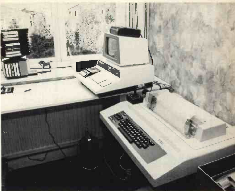
Theodorson's system, showing the printer interface. Pet with extra cassette drive, joystick and printer.
