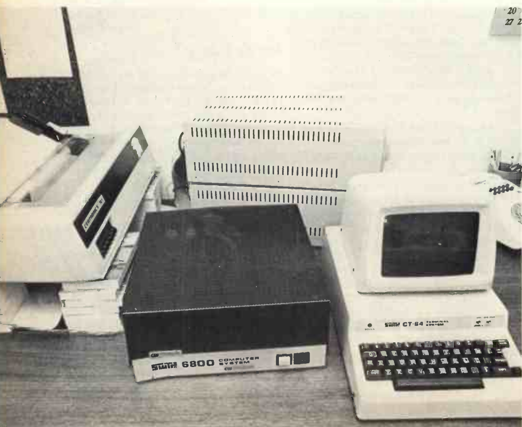
The BUNAC system; 32K processor, twin FD8 discs, printer and VDU.
