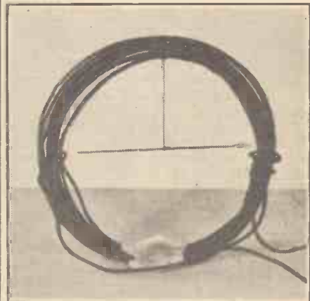
A magnetised sewing needle, suspended from the coil by a short length of silk or cotton, is used in this arrangement.
