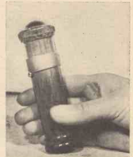
When the rubber band is in this position the flashlamp can be safely carried in the pocket.
