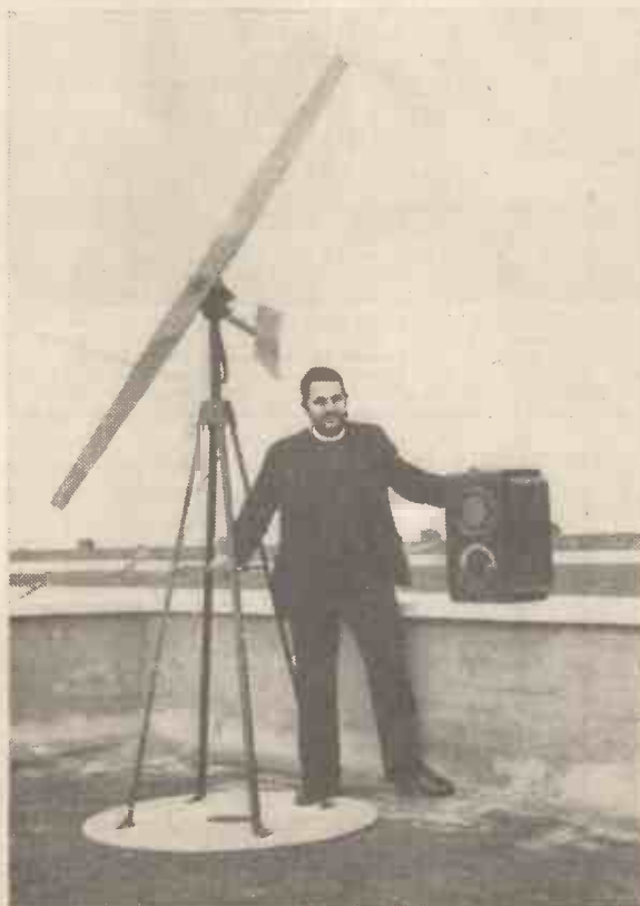
The "Bishop" of Tristan da Cunha with the Ekco receiver he is taking back with him in November. It is a "No H. T." set, being run entirely from the L.T. accumulators charged by the windmill generator.
