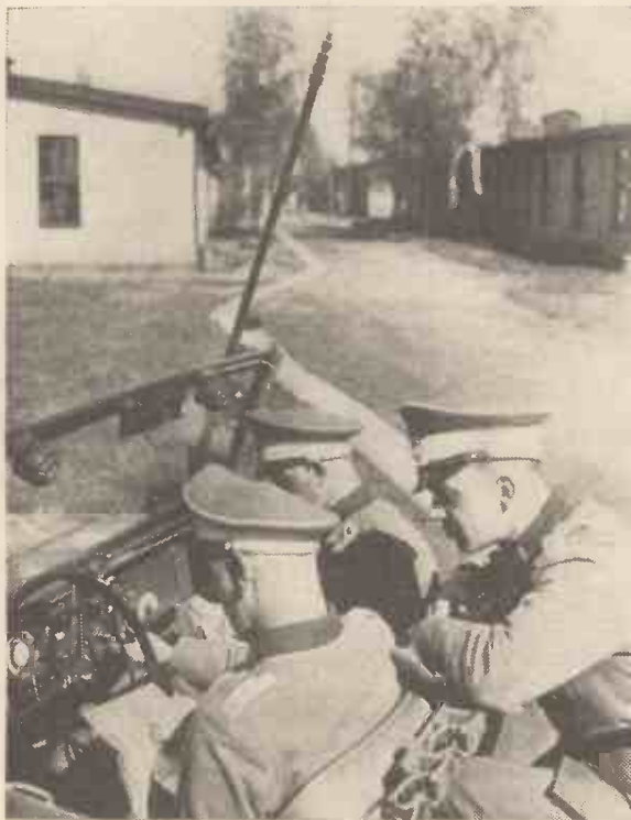
One of the radio equipped cars used by the German police. Note the telescopic aerial which may be extended if desired.
