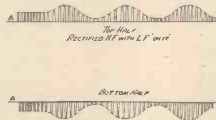
Figs. 4 & 5. The rectified H.F. (top and bottom halves) with the L.F. effect still there.
