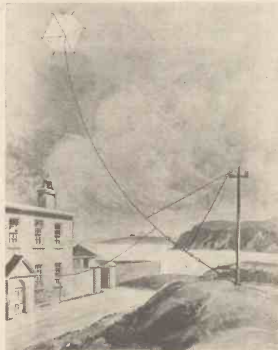
Courtesy Marconi's Wireless Tel. Co., Ltd. A drawing of the kite-suspended aerial, by means of which the first transatlantic wireless signals were received by Marconi, at Signal Hill, Newfoundland, on December 12th, 1901.
