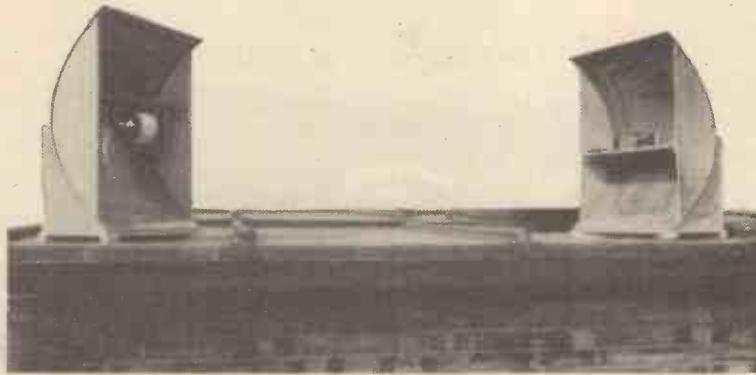
Courtesy, Marconi's Wireless Tel. Co., Ltd. A replica of Marconi's first experimental apparatus which used parabolic reflectors for radio transmission and reception. With such apparatus he demonstrated in Italy, in 1895, the possibilities of beam transmission, and confirmed his results before representatives of the British Post Office and military authorities at Salisbury Plain in September, 1896, when he communicated over a distance of 1½ miles.
