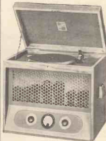
A 60-watt Correx portable amplifier priced at 70 guineas. Provision is made for two microphones, gramophone, pre-amplifier or radio unit.
