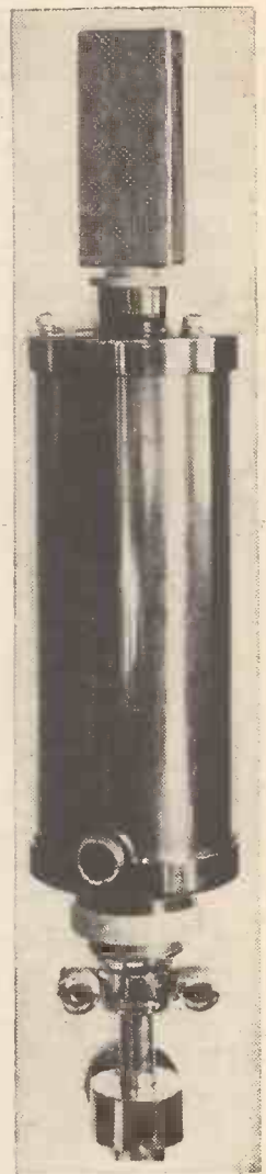
Fig. 1: The Midgley Condenser Microphone and Three-Stage Amplifier. Designed for film recording and studio use, it has an overall gain of 65 decibels. The weight is 8½ lbs.; overall height, 17 ins.; and diameter 3½ ins.
