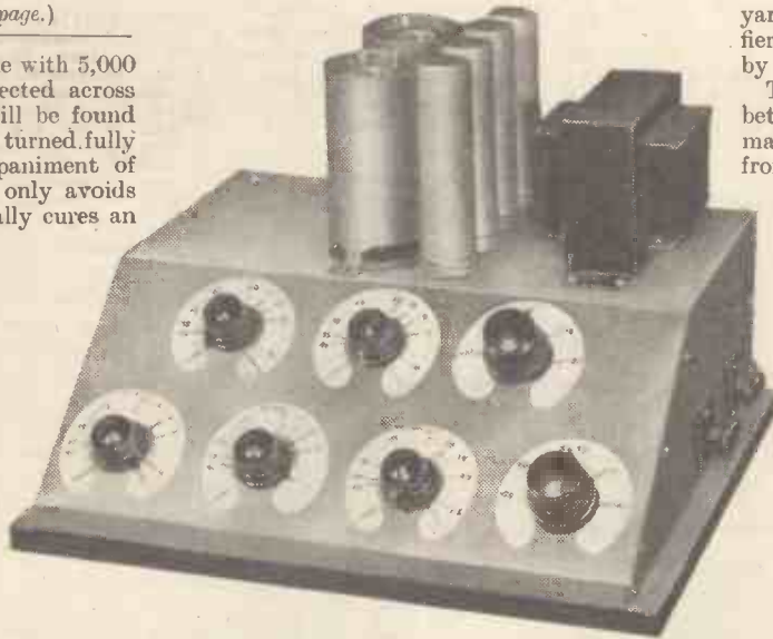
Fig. 4: The completed pre-amplifier unit. The two plugs seen on the right are joined in parallel, so that two amplifiers may be fed from the same unit if desired.
