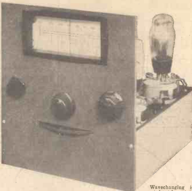
Wavechanging is carried out by rotating the disc which may be seen below the tuning knob.
