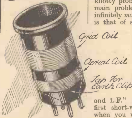
Fig. 1. How a di-pole aerial should be joined up to the aerial coil. Fig. 2 (right) illustrates the method of connecting the earth clip to the aerial winding.
