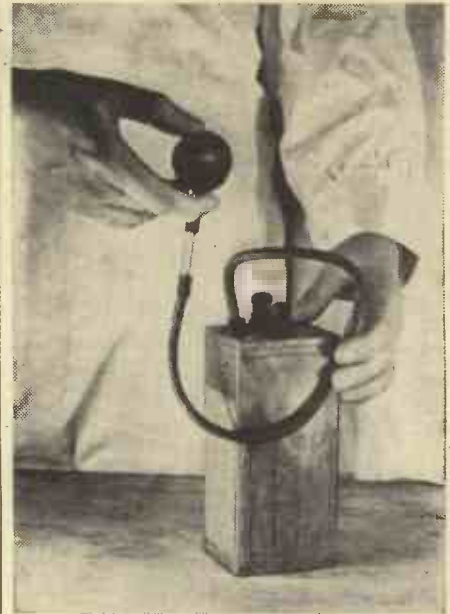
How the tube is inserted through the vent hole of the cell to suck the acid out.
