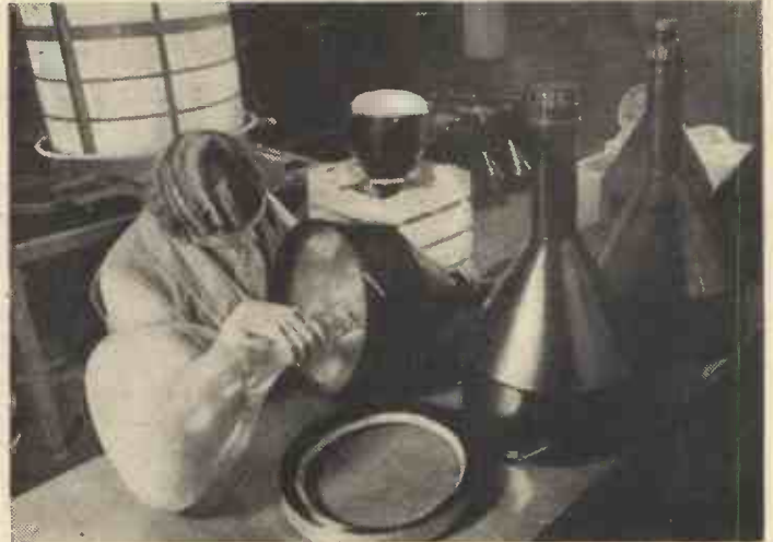
The final stage in the preparation of G.E.C. television cathode-ray tubes. One is seen being fitted into the metal container which protects it mechanically and also acts as an electrical screen.
