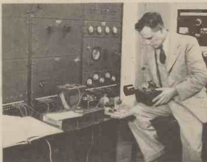
A glimpse of the standard frequency control apparatus at the G.P.O. experimental station at Dollis Hill. A great deal of wavelength checking is carried out here with the object of seeing that the wireless "roads" are kept clear for traffic and that no jamming occurs. Soon this work will be conducted at Baldock, where the necessary apparatus is to be installed.
