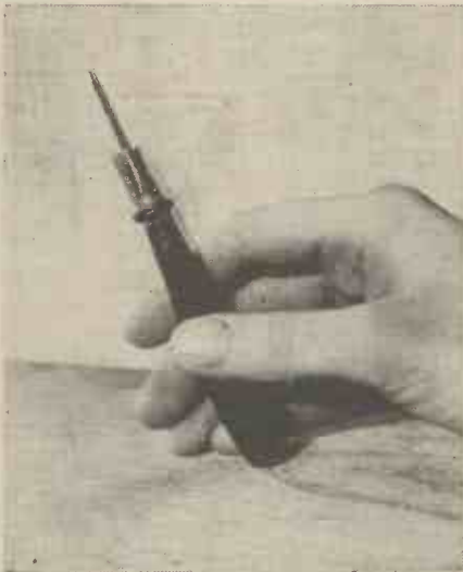
A short length of umbrella rib mounted in a holder as shown, makes a handy tool for cabinet work.
