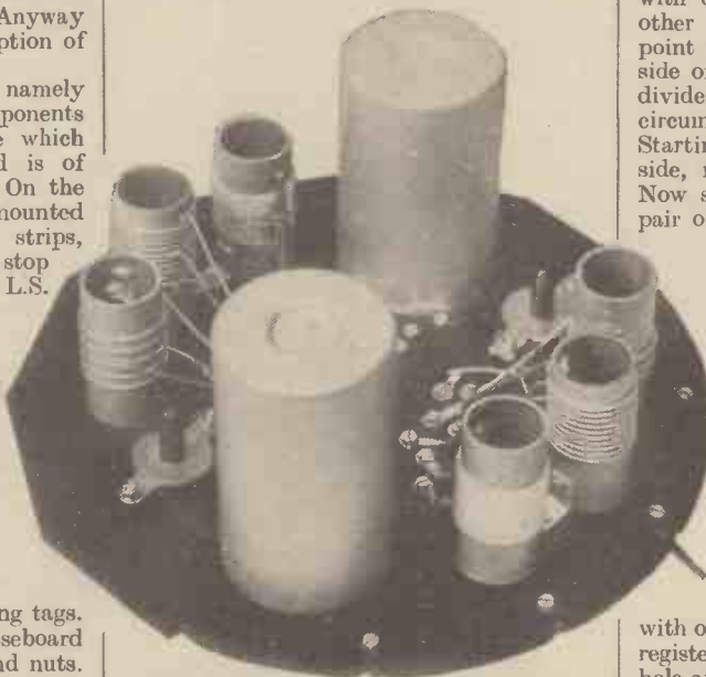
THE COIL UNIT. —The two screened coils are for the ordinary medium and long-wave broadcast bands, while the two groups of three coils cover the short and ultra-short wavebands. These latter coils are home-wound.
