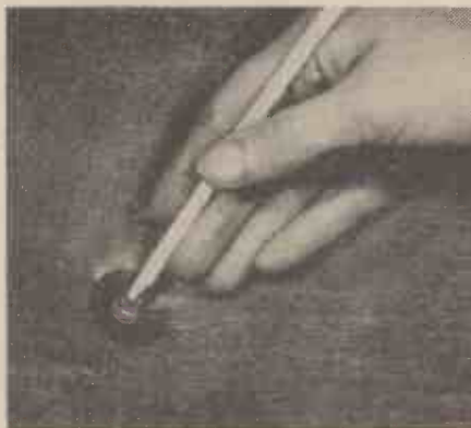
The wax from a taper or candle-end is rubbed well into the exposed threads of the cone bolt.
