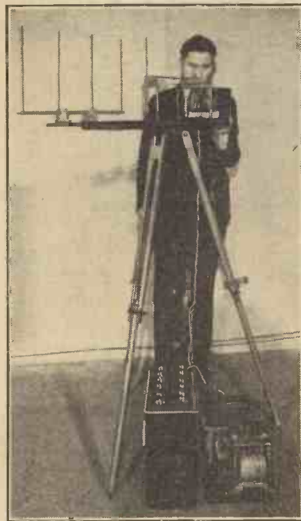
This micro-wave transmitter has a range of ten miles, and has been developed by Baird Television, Ltd., in connection with television. Note the vertical aerial rods.
