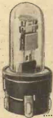
One of the special Marconi "Midget" valves designed for ultra-high-frequency work. The close spacing of the electrodes enables the electron stream to "get across" fast enough to keep pace with the very rapid oscillations employed.
