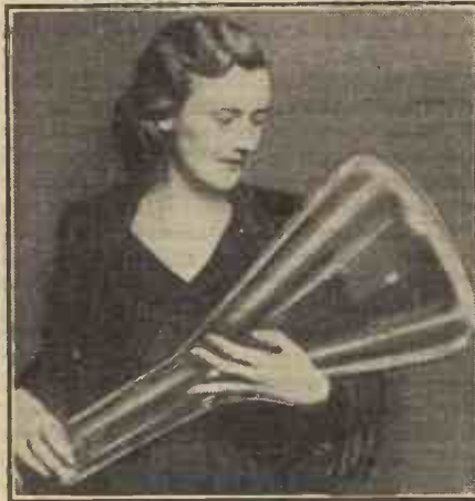
This giant tube is the new Cossor cathode-ray oscillograph which is used in the Cossor television system. It will give pictures nine inches high.
