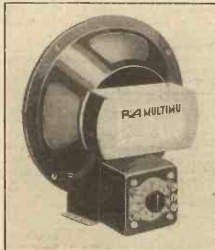
Modern moving-coil speakers are often fitted with a switching device to enable the output circuit to be properly matched up to the output valve.
