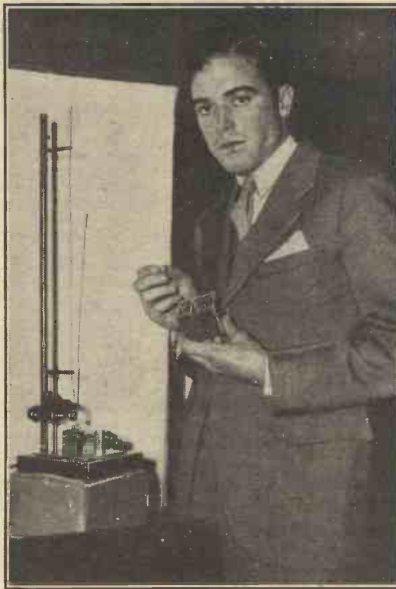
An American firm has recently developed special miniature valves for use in ultra-short-wave apparatus. They are no larger than marbles, and above you see one being fitted to a diminutive receiver.
