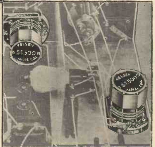
Illustration below shows the position occupied by the Telsen 'S.T. 500' Coils in a built-up 'S.T. 500' Receiver.
