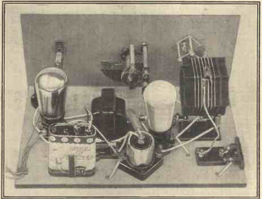
This photograph illustrates the inside of the finished receiver. The detector valve is on the right, while the output stage is to the left. Note that the crocodile clip on the grid coil is located about half-way from the grid end: this will normally be the best position.
