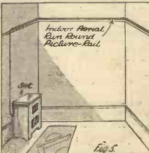
Those who are unable to erect an outdoor or roof aerial should try the arrangement shown above. The aerial wire runs round the picture railing on three sides of the room.
