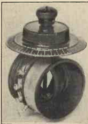
The extent to which the magnetic field set up by one coil can affect another depends upon the relative positions of the coils. By arranging for one coil to rotate within the other the effect of the field can be infinitely varied.
