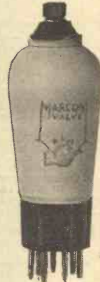
The VP21 was the first battery H.F. pentode to be released. It should prove a very useful valve.
