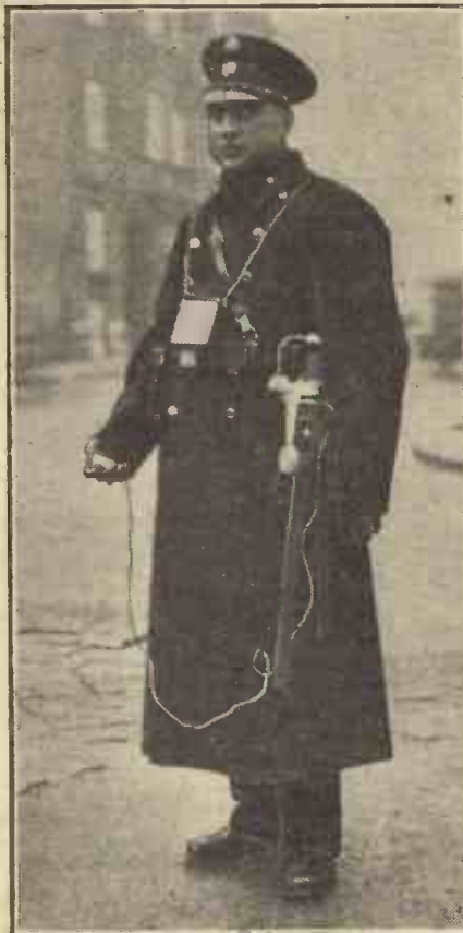
The little box hanging round the neck of this Austrian policeman is a complete transmitter. The battery is contained in one of his pockets, and he is holding a special Morse key in his right hand.
