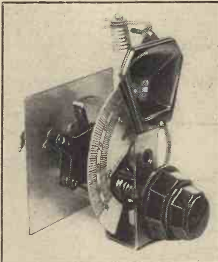
Priced at 10s. 6d., this Magnum double-gang solid-dielectric condenser, made by Messrs. Burne-Jones, Ltd., represents excellent value for money.
