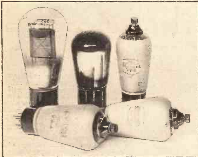
Screened pentodes, large output valves, and double-diode triodes are among the newcomers from Mullard. Here are the D.O.28, the PM 24 M, and three-screened pentodes, V.P.4 and S.P.4.
