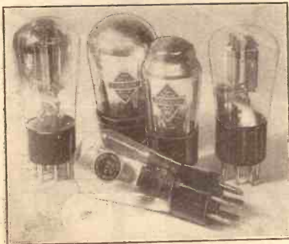
A group of various types of "Class B" valves, including Mullard P.M.2B., Cossor 240B. and 220.B., Mazda P.D.220 and Ferranti H.P.4.
