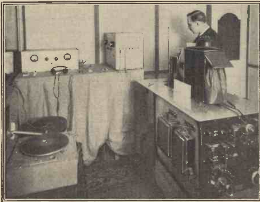
The Baird Television transmitter that was demonstrated during the Olympia Show. The turntable that can be seen on the left is used for supplying gramophone music to fill in intervals.
