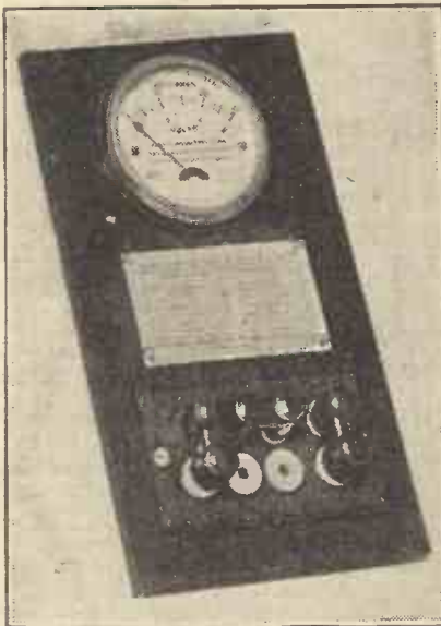
The Wates Panel-mounting Test-Meter fixed on a piece of ebonite to illustrate its layout when in use.
