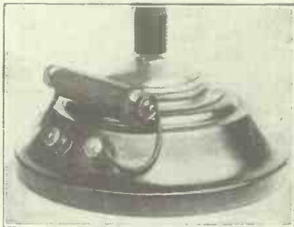
Fig. 1. A permanent crystal detector across the input terminals is well worth trying.
