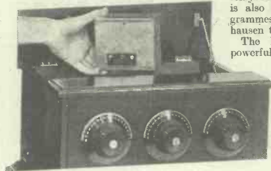
Inserting a wave-trap in a modern set
