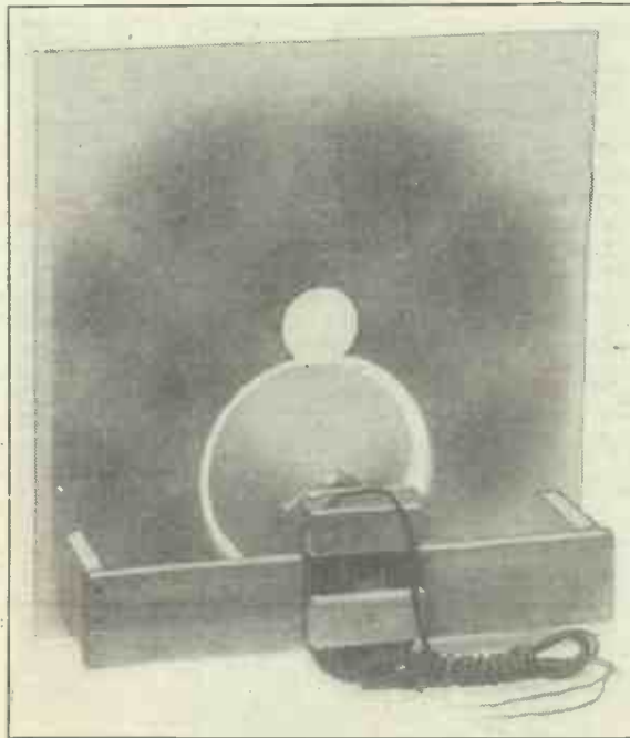
The back of the cabinet removed from the main portion, showing how the supplementary unit is fitted up. The exact position for this unit needs to be determined with a little care to see that it does not foul any of the parts of the main reproducer.
