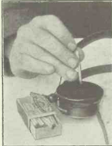
... is best carried out by dropping a match as shown, when the sound will indicate whether or no the diaphragm is free.
