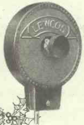
A centre-tapped coil of the type shown here is a great aid to selectivity.
