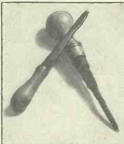
The two screwdrivers insulated as described on this page.
