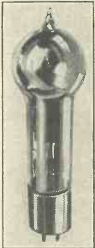
Fig 5.—The Zworykin thermionic photo-electric cell, which combines both the light-sensitive elements and the necessary valve amplifier.
