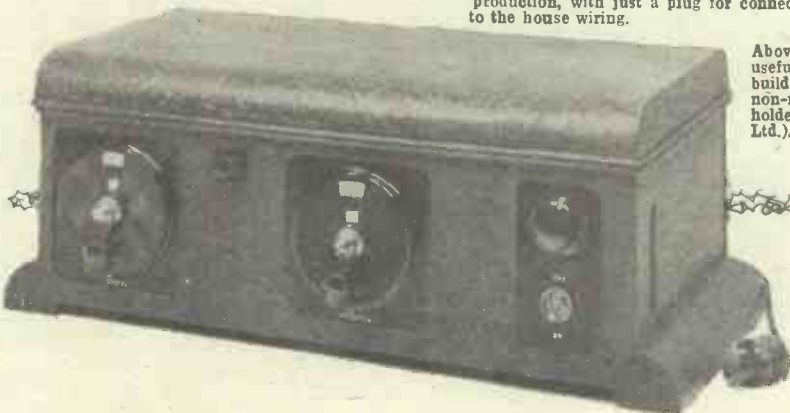
The set of the future will be of the All-from-the-Mains type, with no battery bother at all. That shown below is an "Ekco" production, with just a plug for connection to the house wiring.
