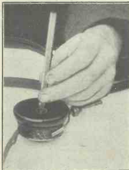
If you wish to test whether the 'phone diaphragm is free or touching the magnet pole-pieces, DON'T tap it with a pencil, as shown. But see page 778.
