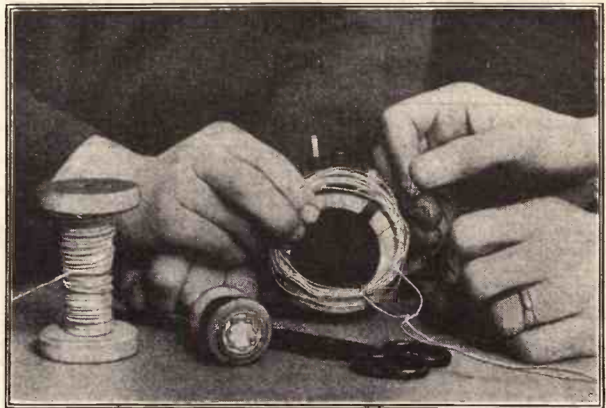
A very high order of selectivity can be achieved in a very simple manner where normally a set has only a single coil, tuned by a paralleled condenser, in its aerial circuit. A few feet of wire (practically any gauge with any covering will do) is roughly wound into coil form and tied to the aerial plug-in coil, as shown above. Aerial and earth leads are then taken to the ends of this new coil instead of the set. The bigger the coil the less the selectivity attained. Twenty turns is an average number.
