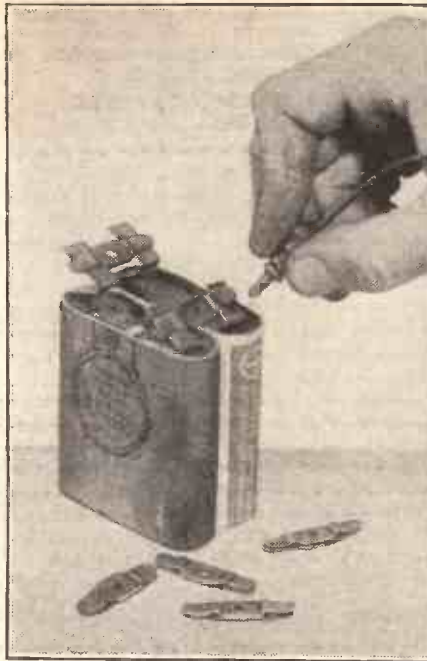
The long strip of the flash-lamp battery is the negative terminal, and the short strip is positive. To connect two batteries "in parallel" the like strips are joined together. The total voltage remains the same (4½v.) but the capacity is doubled.
