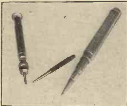
On the left is shown the small screwdriver adapted as a scriber and centre punch. In the centre is a centre punch made from a small round file and on the right is the other form of scriber dealt with in this article.
