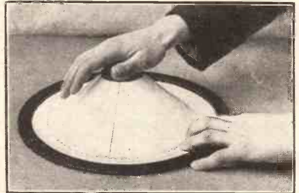
Sticking the edge of the cone to the suspension leather. Be careful to press all the little serrations down into proper adhering contact.
