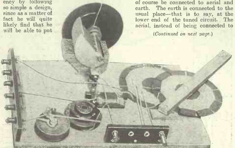
Three tappings are arranged for the aerial coil and are connected to the three sockets shown on the right of the small terminal strip.
