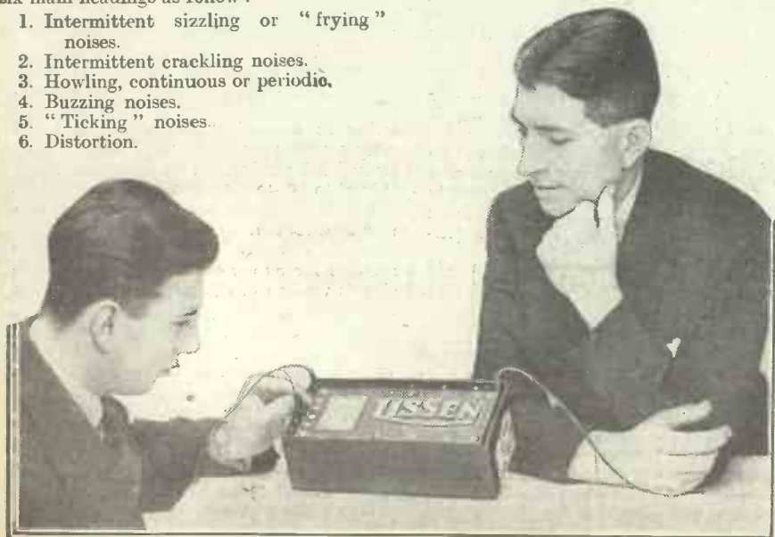
Even the best of H.T. batteries will run down after a long and useful life, and need replacing if good results are desired. But the contacts between the wander plugs and their sockets should be checked up and cleaned periodically in order to avoid wrongfully suspecting the battery of "making noises," when actually it is in good condition.
