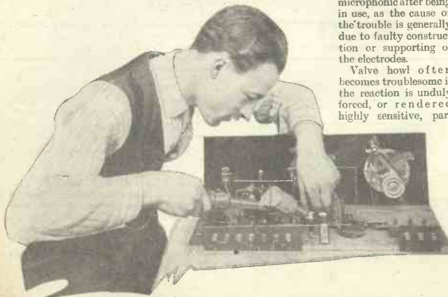
This constructor is using an electric soldering iron, but few amateurs possess such a luxury. With one of these useful articles clean and efficient joints are easily made, but an ordinary soldering iron carefully handled can do just as good work even if it takes a little longer to do so. Faulty joints cause a great deal of trouble in radio receivers.
