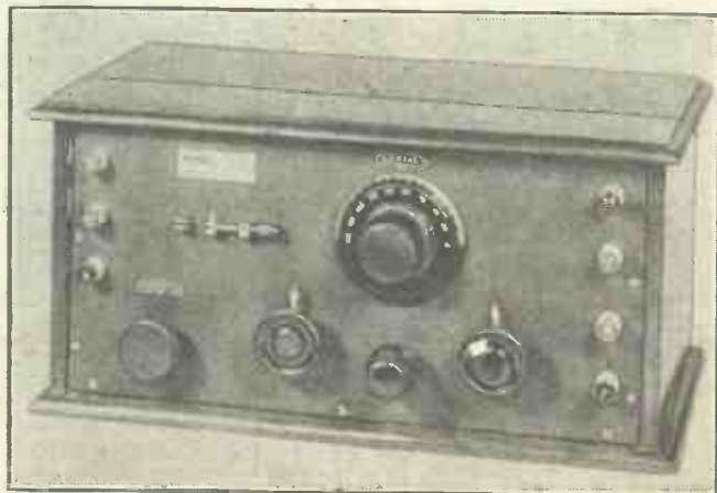
The most popular of four-electrode valve receivers—a two-valve Unidyne.
