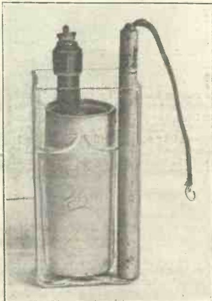
Fig. 2.—This is the complete Barber cell, which is stated to have considerable possibilities.
