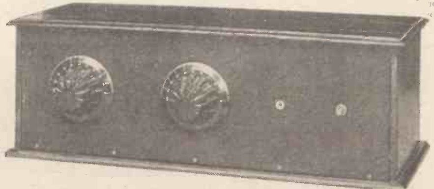
The panel lay-out is pleasingly simple. The small object between the right hand condenser and the on-off switch is a bushed "window" intended to enable the operator to see whether the valves light. Since so many modern valves give little glow this is to be regarded as an optional fitting, and is therefore not marked on the diagrams.
