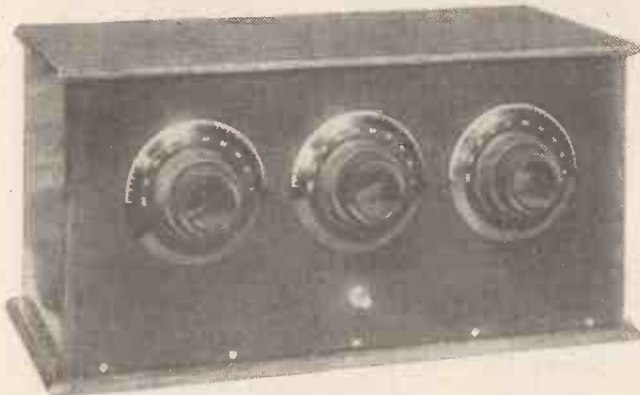
This is the complete set. The three dials from left to right, are the two tuning condensers and the reaction control. A switch for switching the set on and off is the only other panel-mounted component.
