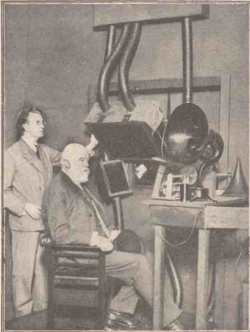
Mr. Baird showing Sir Oliver Lodge how his Noctovision apparatus operates in conjunction with the Television system.
