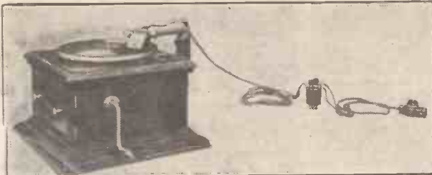
The Igranio-Phonox "Phonovox" fitted on a gramophone and complete with plug for insertion in a receiving set.
