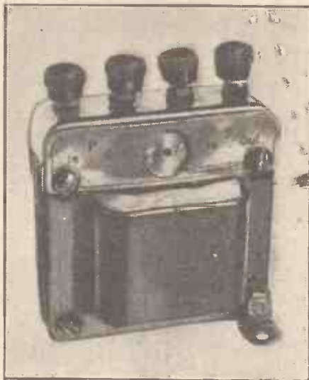
Fig. 2.—A typical shrouded L.F. transformer.
