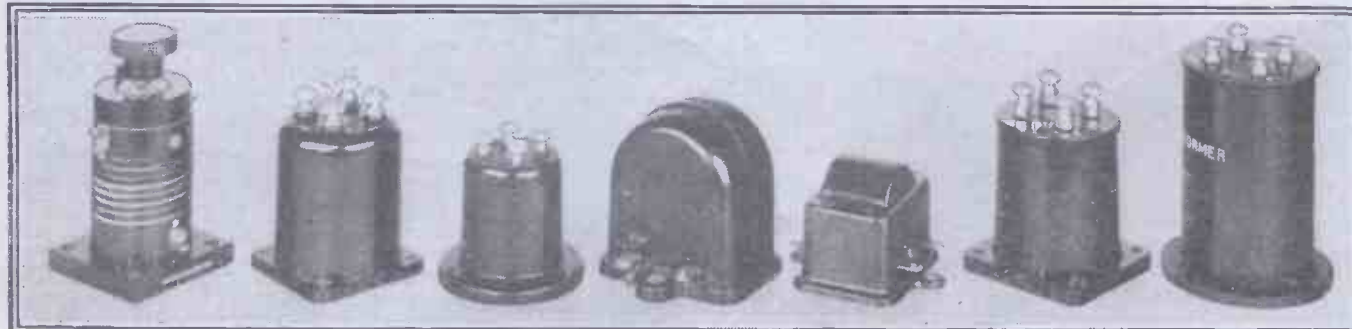
A few of the types of super-heterodyne intermediate transformers used in my experiments. Some are British, some American.
