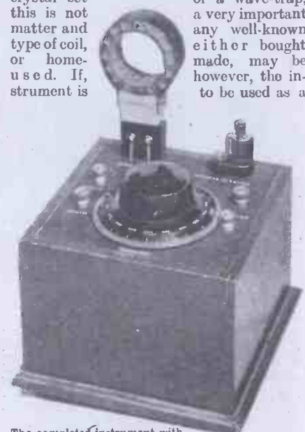
The completed instrument with plug-in coil in position—ready for use as a crystal set.
