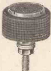
Showing Crystal partly removed from cup.
