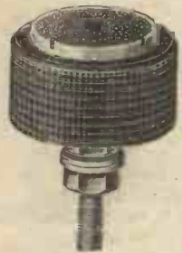
Showing Crystal partly removed from cup.
