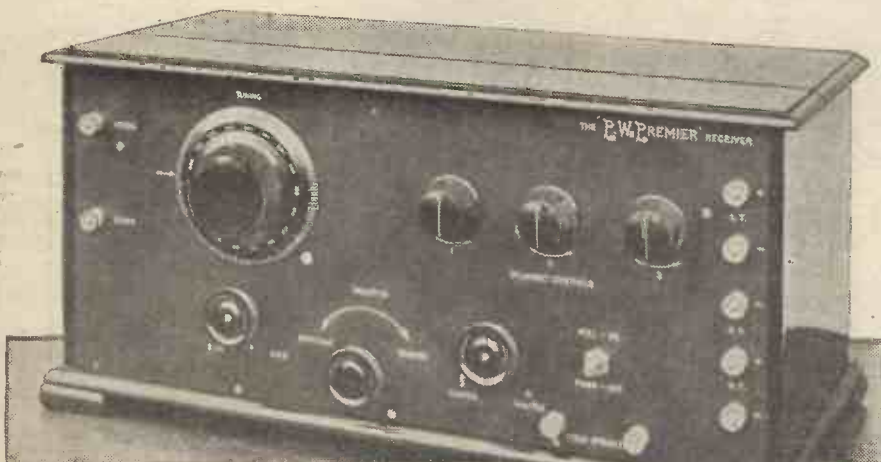
The handsome appearance of the "P.W." "Premier" receiver strikes a distinctive note in radio design. The controls, as shown by this photograph, are arranged both symmetrically, and so that tuning operations are facilitated.
