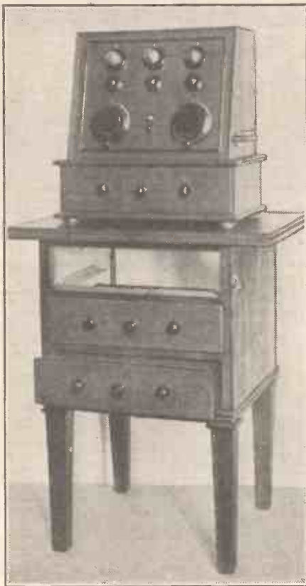
A German cabinet receiver, recently designed to cover all wave-lengths between 200 and 3,000 metres.
