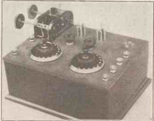
A photograph of the completed receiver taken before the transfers were placed on the panel.
