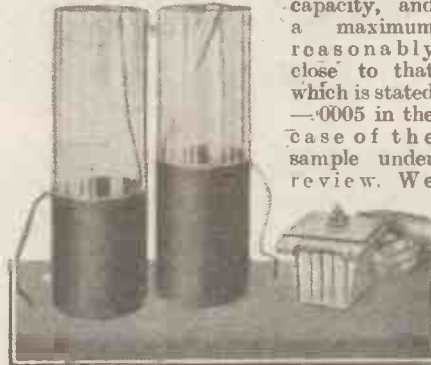
Two Leyden jars compared with a Dubilier Standard Mica Condenser. The latter has a capacity equalling the two "jars," but is more efficient and more electrically robust.
