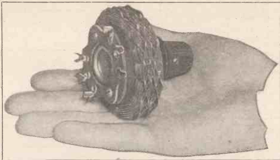
The desire for compact radio components has resulted in this complete three-circuit tuner recently introduced in America.
