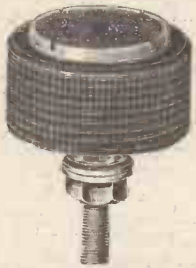
Showing Crystal partly removed from cup.
