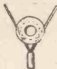
Divide your wire, pass it round either side of the eyelet, and twist the ends together.
