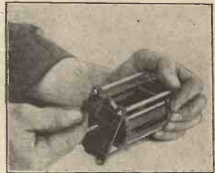
Fig. 14. Winding the stator.
