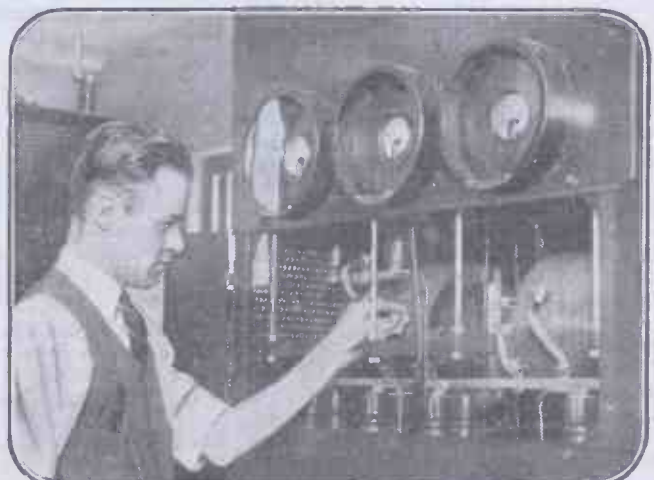
Adjusting W J Z, the new American broadcasting station, to 455 metres.
