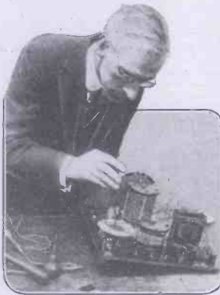
Fixing in the anode coil. The "P.W." Combination Set in the course of construction.
