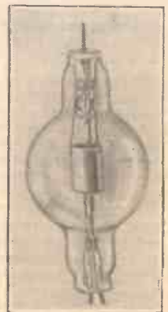
A modern three electrode thermionic valve.
