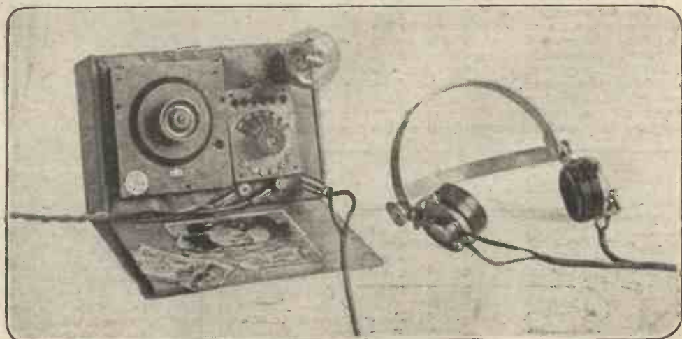
A very compact and, considering its size and genus, very effective cigar-box receiver, made by Mr. J. McCallum, 11, Avenue Mansions, North Side, Clapham Common. The set will receive clear signals and speech from several high-power stations without any outside aerial at all.
