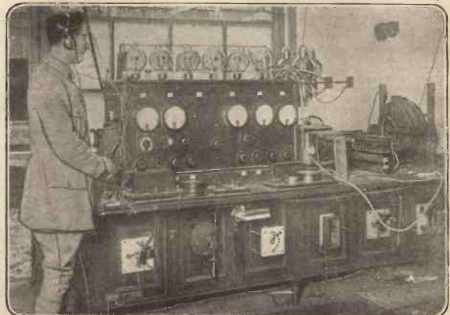
This telephony-transmitting set has been temporarily installed at the Eiffel Tower, and amateurs are familiar with the speech and music sent out by it every evening. A larger and more powerful telephony transmitter will shortly be installed.
