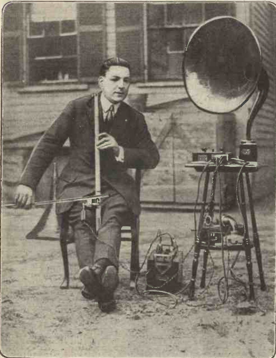
A one-man broadcasting station in America. The instrument is of the one-string variety, and is played upon with an ordinary violin bow. A microphone is attached to an ordinary gramophone diaphragm to reproduce the louder tones.
