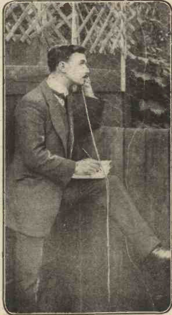
You can enjoy plenty of wireless "stunts" if you live near a wireless station. This Croydon resident uses a wire fence for an aerial and an accommodating dustbin for an "earth."
