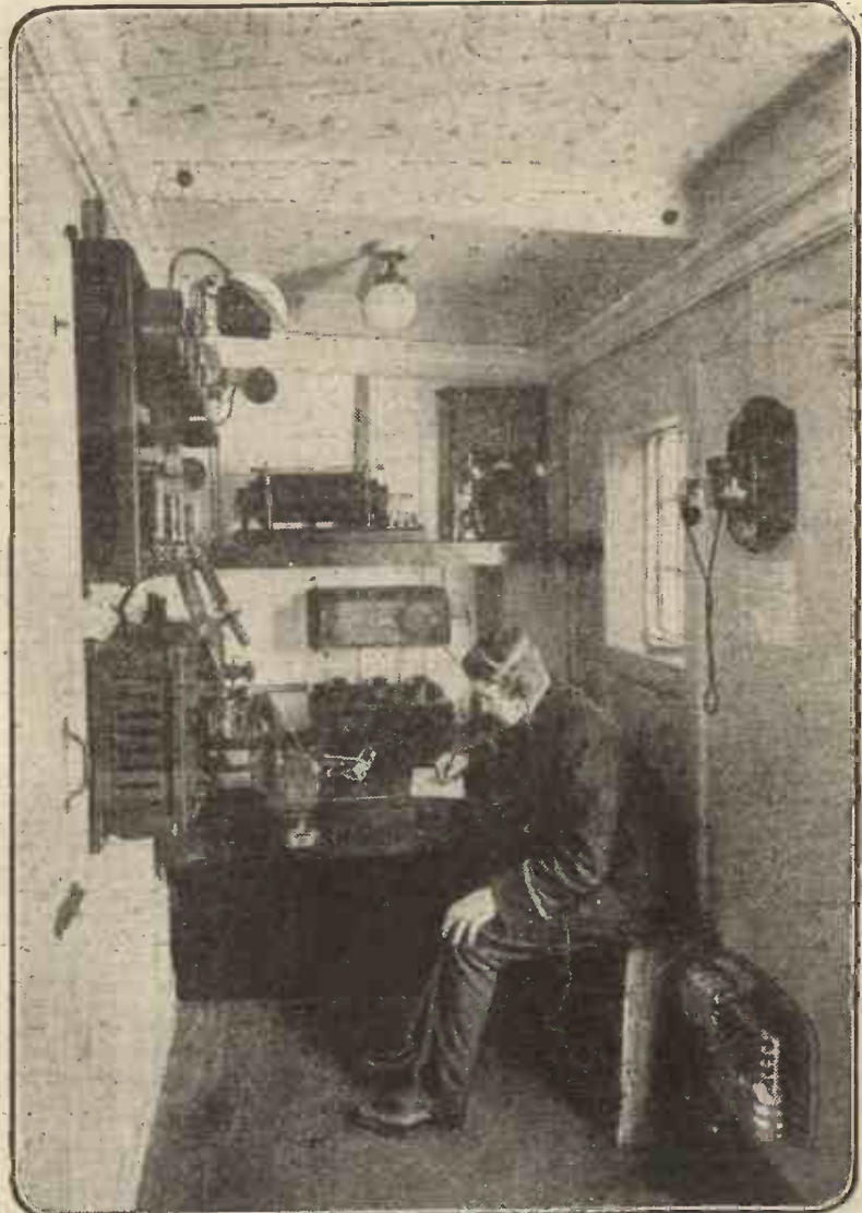
This photograph shows the interior of a wireless room on board a ship. The old magnetic detector, with the glass case front and the multiple tuner directly beneath, are used as an emergency receiver, the crystal detector being placed on the left of the table. The emergency 10" spark coil is also shown.
