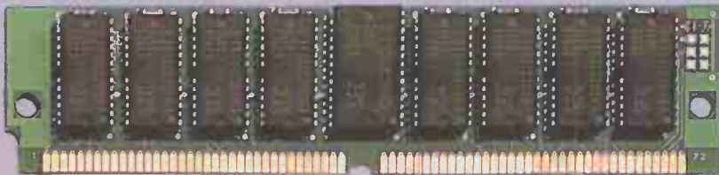
72 PIN SIMM ACTUAL SIZE. CHIP CONFIGURATIONS MAY VARY.
