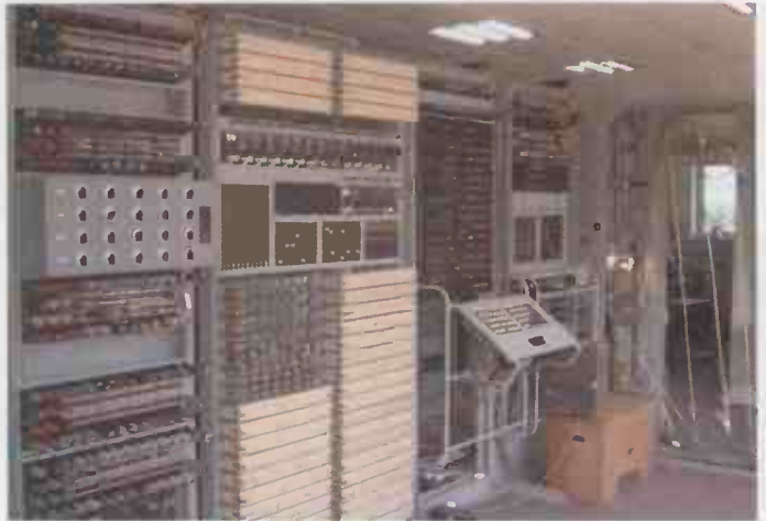
The Colossus, the world's first digital electronic computer, could break German codes varying up to 10^{18} combinations, all with vacuum tubes. Not bad hitting for the first of its kind!
