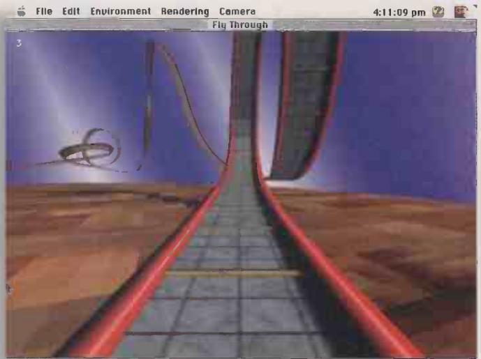
This early demonstration of Quickdraw 3D features texture mapping and complex shading. The image is updated in realtime as the camera moves smoothly along the rollercoaster track
