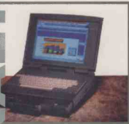
The Acer Note Pro notebook is one of several new models with a built-in touchpad
