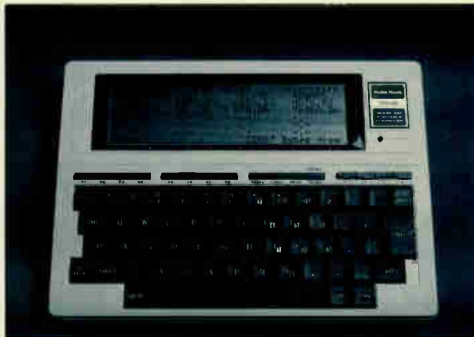
The Tandy's striking feature is the 40 character by 8 line display
