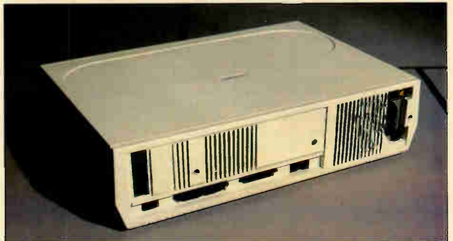
Pop out panels at the back allow sockets for add-on interface cards.
