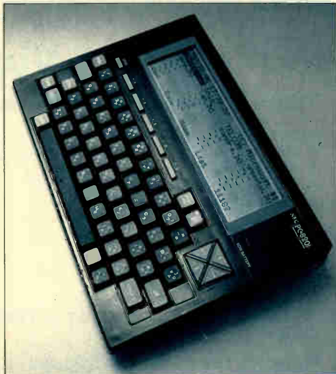
The NEC 8220 has two memory boards totalling 64kbytes
