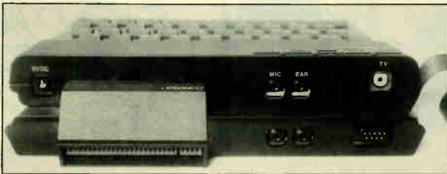
The interface slots into the edge connector at the rear.
