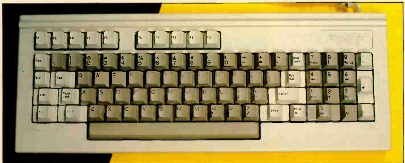
Keyboard layout is IBM PC compatible with 84 keys including 10 function keys and numeric keypad
