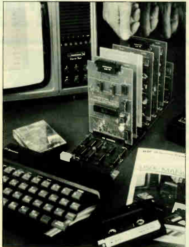
An expansion for the ZX Spectrum: U-Microcomputers has designed an extension of the system bus that takes several extra circuits.
