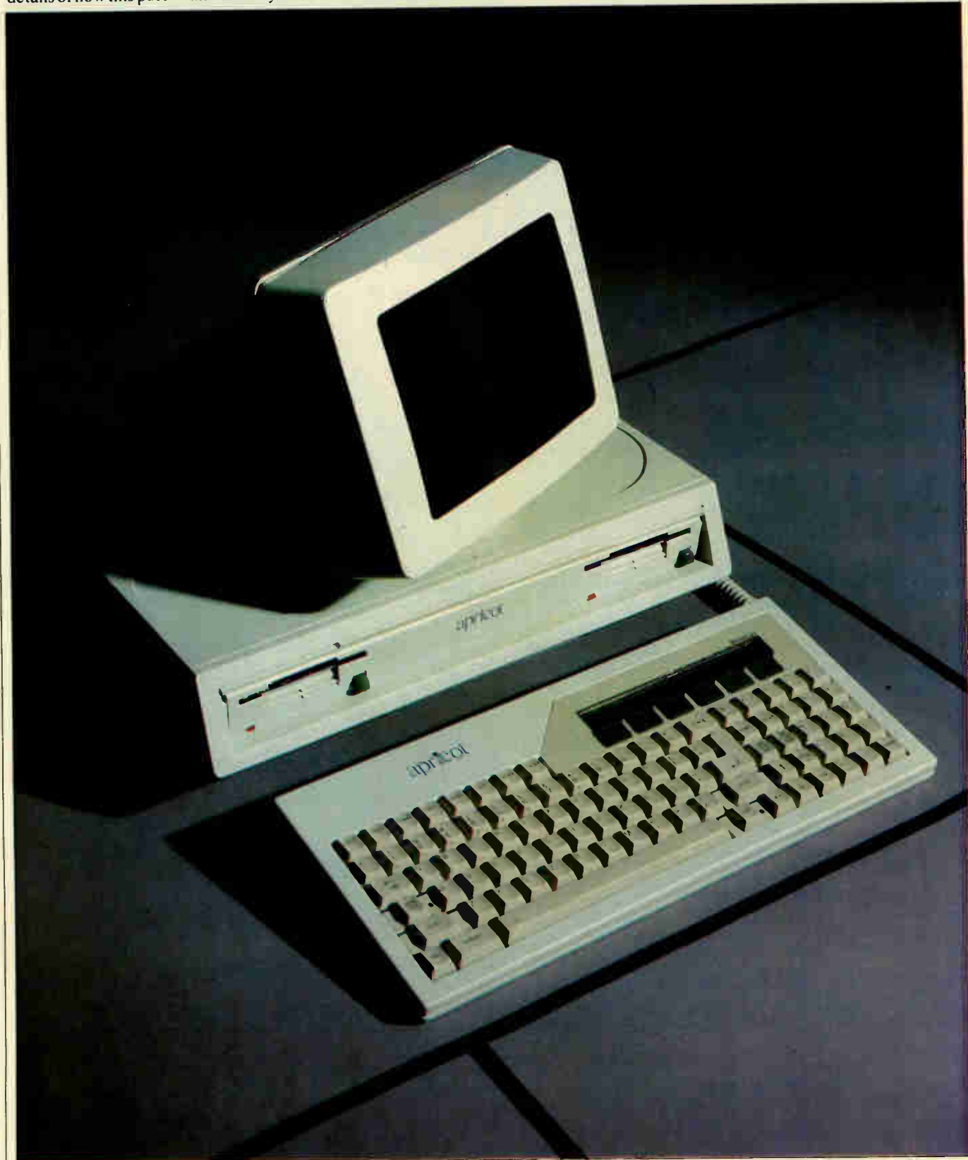
The 'transportable' Apricot is precisely and expertly designed with the keyboard clipping neatly to the underside of the main box.
