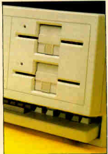
Keyboard slots into a shelf under the display and diskettes
